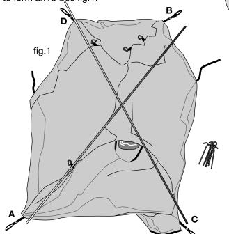
• Insert the first pole post into the grommet on the corner stake-out web at A. See fig.2. At the opposite corner, B, grasp the web and simultaneously push the pole to form and arc. Insert the locking end tip into the grommet at **B**. Repeat with the second pole section at
